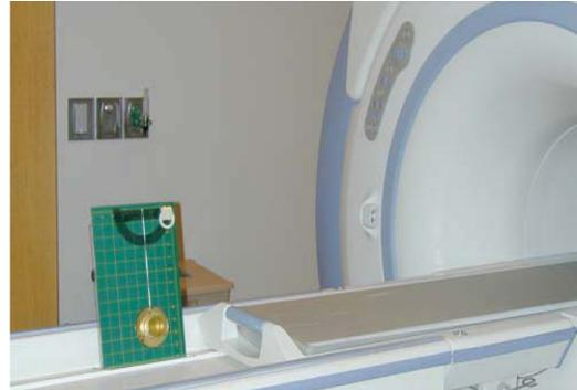
*Figure 2. Set up for deflection angle testing of sprinkler.*
