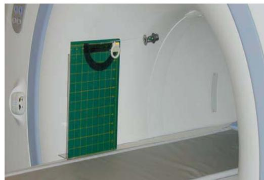
*Figure 4. Sprinkler with small deflection angle and, thus, low magnetic field interactions.*
