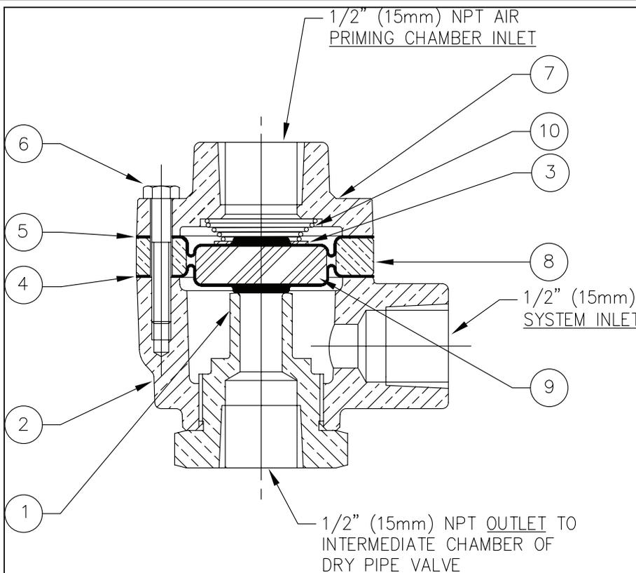
**Figure 1: Model B-2 Anti-Flood Device for use with VdS Approved Model E-1 Accelerator Trim ONLY**
